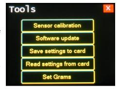
**SENSOR CALIBRATION:** Sensors are already calibrated in our factory. In case the sensors require recalibration, this button provides access to the calibration procedure.
