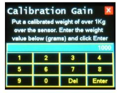
It is always recommended to calibrate all 3 sensors at the same time, so that all 3 are calibrated with same reference weight. Differences of calibration between sensors will
