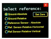
The Side Buttons allow selecting the reference for the measurements.
