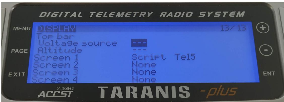
After that head to the main screen and long press the “Page” button. If all the process is done correctly the Xicoy telemetry screen should appear.
