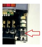
The last step of the pairing procedure is to confirm that you own the adapter that is being paired, to prevent the possibility that another person could link to your ecu and modify the settings. The BT adapter has a small button close to the green led.
