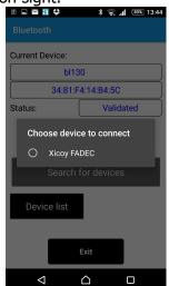
When the operating system on the phone finishes the pairing procedure, the app will ask you to confirm that you own the adapter being paired. Press the button on the adapter within 30 seconds after the message appears.
