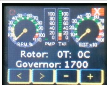
Governor. The next screen is for the Heli and shows the governor setting for rotor head RPM. **Default is 0 meaning OFF.**
