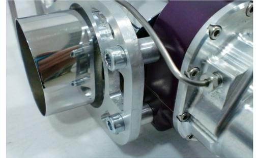
Note the solid fixing of the gearbox to the mounting and through to the firewall, critical in providing a stiff, yet load sharing pathway. This simple but rigid framework provides a lot of engine protection in event of a nose over or crash, however this stress will be passed directly to the firewall so must be a secure point in the airframe.
