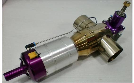
The unit is designed to operate with the output shaft uppermost. A side and plan view can be downloaded from [www.Xicoyturbines.com](http://www.Xicoyturbines.com). Use the link to check for other sizes of mounting and views to suit specific airframes as they become available.
