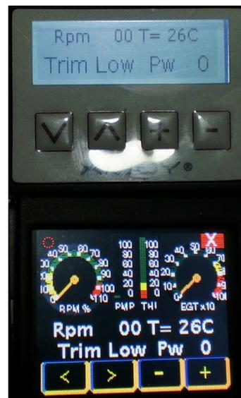
Both displays include dedicated screens for engine operation, radio checking, last shutdown cause and other special turbine operations.
