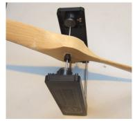
**Important** - No attempt should be made to add material, lead shot or coloured sticky tape to balance the prop as this is sure to fly off later and if you are lucky it might not to hurt someone, but the resulting out-of-balance running could cause major engine damage. If this happened in the air you would not know until it was too late. The warranty will not cover you for such damage.
