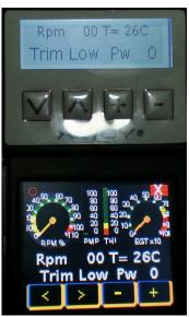
Playback mode can be still, forward or reverse, speed x1, x 10 and x100 in both directions, so can be easy to view the engine operation or investigate any issue at the field without the need of a computer or any other type of reader.
