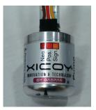
Note: the three wires are <u>NOT</u> for the 3phases usually used for a brushless motor. The three wires are for the plus and minus power supply, and a single wire bidirectional digital link.
