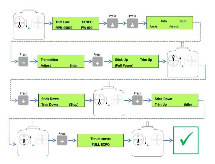
The correct adjustment of the throttle adjustment on the ECU can be verified in the second screen of the display as used before. The percentage of the throttle position should read 0% at the position of engine stop (trim and stick down), 100% with stick/trim full up and between 10% and 30% at idle.
